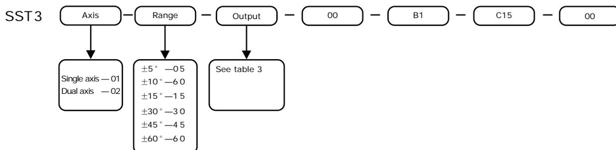
For example, if order a dual axis thermal shock-proof inclinometer, with range  $\pm 15^\circ$ , room temperature accuracy  $\pm 0.02^\circ$ , output RS422, 2 meters cable with plug, the model should be chosen as: SST302-15-G2-00-B1-C15-00
