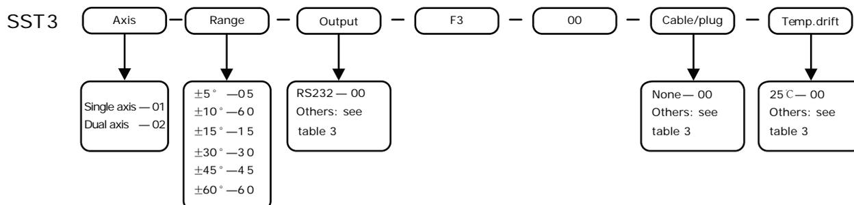
For example, if order a Ranged inclinometer, with range  $\pm 15^\circ$ , room temperature accuracy  $\pm 0.02^\circ$ ,  $-20$ – $60^\circ\text{C}$  accuracy  $\pm 0.02^\circ$ , two meters cable with plug, the model should be chosen as: SST302-15-00-F3-00-C11-D3(2m) .
