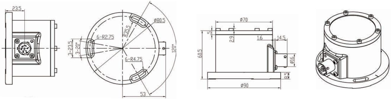
Picture 1 Housing with MIL class connector
