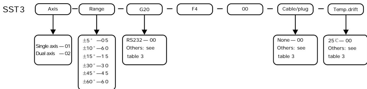
For example, if order one Gyro-inclinometer, with tilt range ±60°, dual axis, absolute tilt accuracy±0.08°, -20~60C tilt temperature compensated accuracy ±0.02°, X & Y axis gyroscope(X axis range ±100°/s, Y axis range±250°/s), 2m cable with plug, 0~5VDC output, the final model should be chosen as : SST302 - 60 - G20 - F4 - 00 - C1 - D3(gyroscopes with X axis range ±100°/s, Y axis range ±250°/s)
