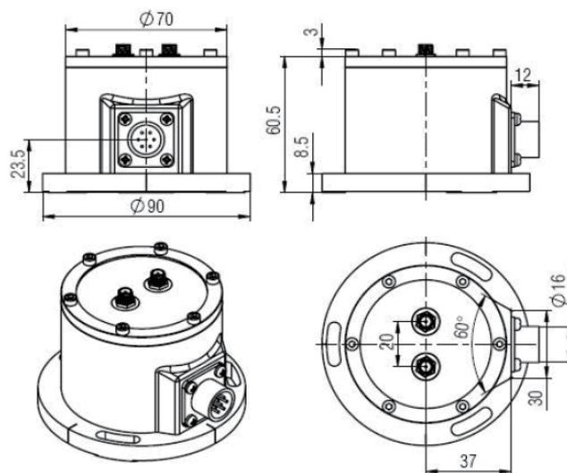
Picture 2 Housing with MIL class connector
