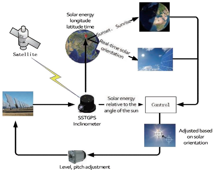
Picture 1 GPS inclinometer in solar energy automatic control application
